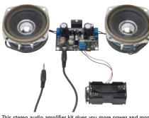
This stereo audio amplifier kit gives you more power and more volume than our standard kits. Each channel can deliver up to 10W for a louder, crisper sound. The kit is supplied complete with speakers. Supplied with assembly instructions
