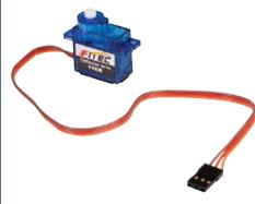
The FS90R is an analog micro servo that is capable of continuous rotation clockwise or anti-clockwise, as opposed to moving to a set position. The servo is ideal for the beginning roboticist and is perfect for use with the Motor Shield for Arduino. The servo can be controlled using any servo code, hardware or library and to control with an Arduino, just connect the orange control wire to pin 9 or 10 and use the Servo library included with the Arduino IDE.
