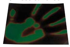
A self-adhesive 150 x 150mm sheet printed with a thermochromic liquid crystal ink which changes colour when heated above 27°C.
